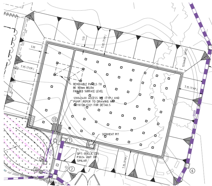
Plan drawing of the dual tank system
